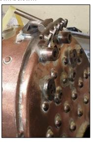
The everlasting blowdown valve is as drawn by Don. There are two extra water feed bushes along the bottom of the backhead, one of which will be used to fill the boiler using a HP electric pump, this will be able to feed water against boiler pressure if ever required, something I doubt will ever be needed but it's nice to have a backup when there's no hand pump in the tender which according to Don would be undignified to have on this loco, I agree.
