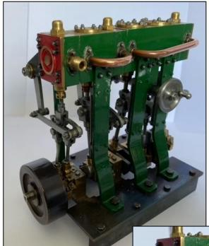
build up initial pressure in all cylinders before the double or triple will turn over properly.
