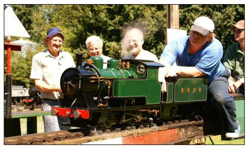
Romney Hythe and Dymchurch Railway by Kraus in 1926. The original engine left Kent in 1933 and ended up in a Belfast scrap yard, brought back to the RH&DR and was restored in the mid-1970's. During the restoration two 5" models of this engine were built alongside and one of them visited us with members of the Maidstone Club in 2007. The engine has unusual outside Stephenson link motion.
