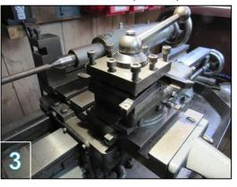
actual machining all the assorted components takes some time, of which more later. The design is actually for the ML10 lathe, but it is suggested that it could be adapted to suit larger lathes and this is what I have done, by fitting a raising plate underneath the toolholder itself.
